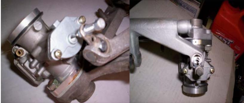
Remove the stock rubber grommets from the air filter box. Stretch the O rings provided over the carburetor inlet mouth. The air filter will be closer to the carburetor body and make up the difference in length of the JRC carburetor. Install assembly on the bike and complete fuel line fabrication.
