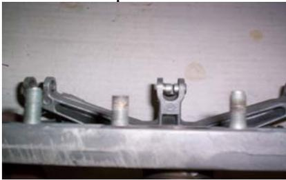
You will need to remove 1/16 inch from the left carburetor retaining stud as shown. Thread one of the nuts on the stud and grind the stud. Remove the nut to remove any burrs on the stud left from grinding.
